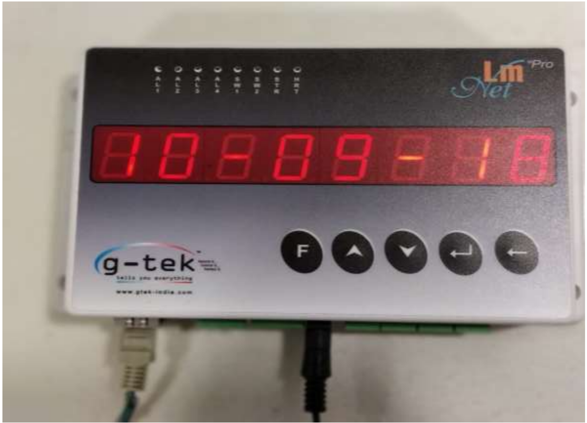
Figure 6 LmNet connection with Adaptor and LAN Cable
