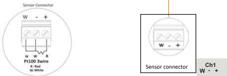
Figure 10 Sensor Wiring - RTD 3 Wire input
